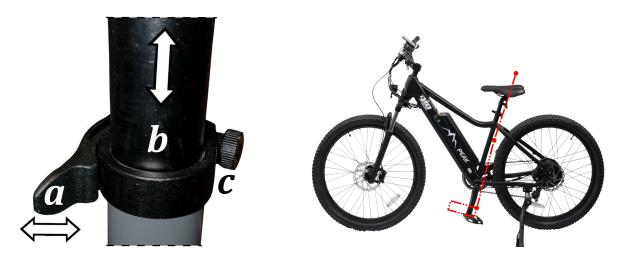
Always ensure your seat is correctly positioned, this can be achieved with the following simple method. Lower one of the pedals into a position that aligns its crank arm with the seat post, then place your heel on the pedal. A seat at the proper height should create a straight leg while seated in this position. (See pg07 picture) This alignment will provide the most power and proper range of motion for the joins responsible for pedaling your e-bike.
