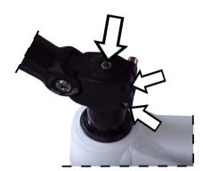
The angle of the handlebars can also be adjusted by loosening the bolt securing it, making the desired adjustment and retightening the bolt.
