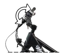
Suggested torque for the handle bar fasteners is 13-14Nm. Reflectors on the handlebars may need to be adjusted due to movement during shipping. You may need to loosen, adjust and retighten once the wheel is installed to ensure proper alignment.
