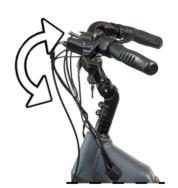
Suggested torque for the handle bar fasteners is 13-14Nm. Replace the rubber plug in the stem when alignment/tightening is complete. Reflectors on the handlebars may need to be adjusted due to movement during shipping.
