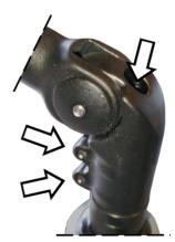
The angle of the handlebars can also be adjusted by loosening the bolt securing it, making the desired adjustment and retightening the bolt.
