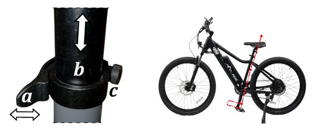
Always ensure your seat is correctly positioned, this can be achieved with the following simple method. Lower one of the pedals into a position that aligns it's crank arm with the seat post, then place your heel on the pedal. A seat at the proper height should create a straight leg while seated in this position. (See picture above) This alignment will provide the most power and proper range of motion for the joins responsible for pedaling your e-bike.
